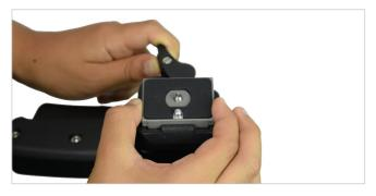
Attach the tripod plate to the base of the IKE device ensuring it is positioned correctly as shown below. Tighten the screw until it is secure.
