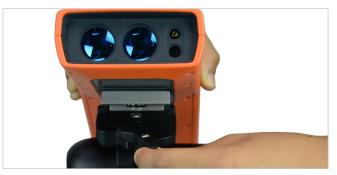
Lower the IKE unit into position and then turn the lever fully to lock the unit into place.
