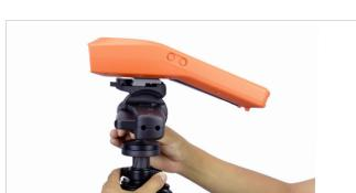
To adjust the position of the IKE device, with one hand hold the unit, and with your other hand squeeze the main lever and move to adjust.
