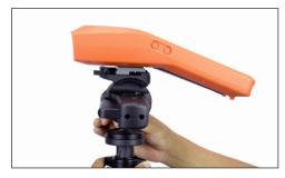
You can fine tune the height of the unit. Turn the adjustment ring counterclockwise to loosen it and lift the center pole. Turn the adjustment ring clockwise to tighten into place.
