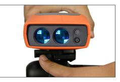
Lower the IKE unit into position and then turn the lever fully to lock the unit into place.
