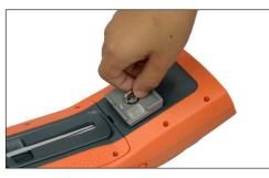
Attach the tripod plate to the base of the IKE device ensuring it is positioned correctly as shown above. Tighten the screw until it is secure.
