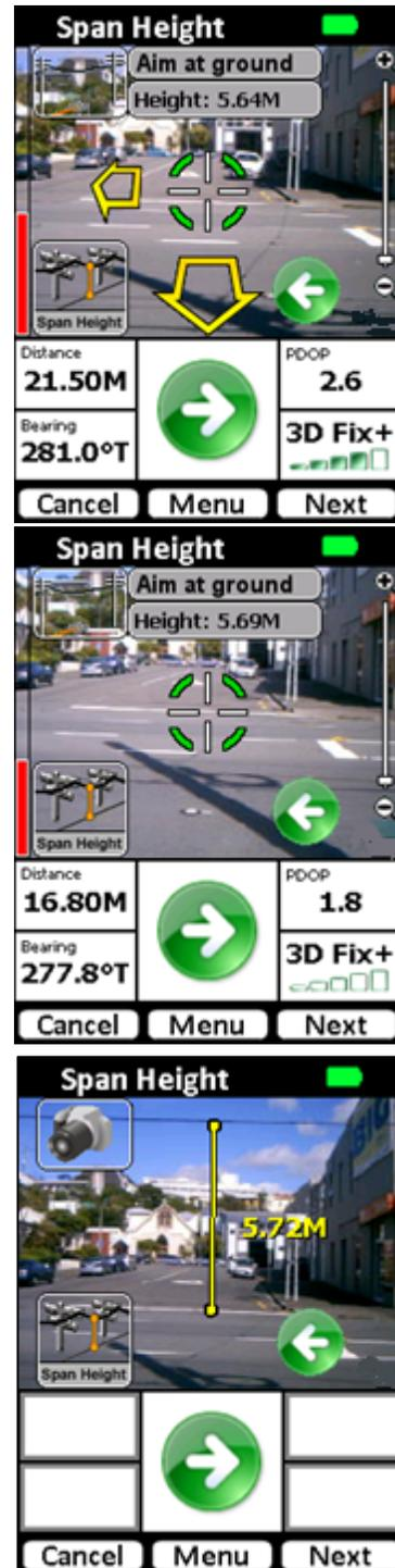
The camera will click, and depending on camera settings, will revert to the Span Height selection screen. Where there is a successful recording a green tick will appear alongside the task.
