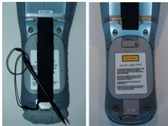
Unlock the battery cover by sliding the lock to the right.
