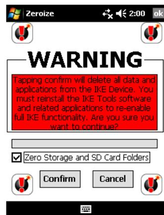
After Zeroize, IKE OS must be re-installed to restore full IKE functionality. Any other applications that were previously installed on the IKE unit must also then be manually reinstalled to return that functionality.
