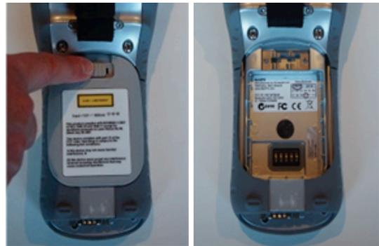
Place the battery into the battery cavity
