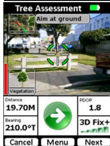
Aim the IKE at the trunk of the tree to mark the DBH (diameter at breast height) and tap the Next (green arrow) button.
