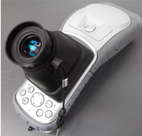
Incorrect placement of Glare Shield
