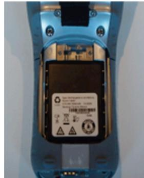
Replace and secure (slide the lock to the left) the battery cover
