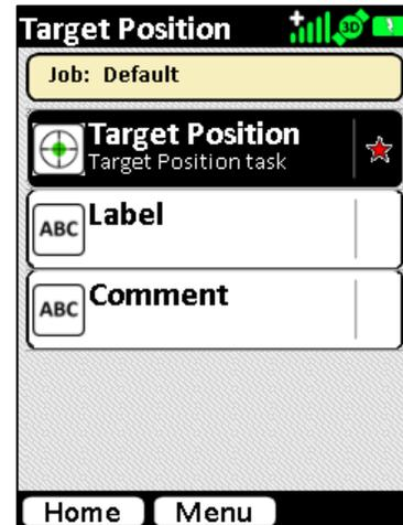
Move your IKE until the crosshairs are centered on the target object you wish to capture data on. Check that the PDOP and GPS Fix readings are good. The border around the instruments readouts will change in color depending on the quality of the reading.
