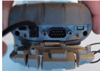
The red power/charge LED should light/blink if power is correctly applied
