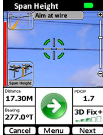
Aim at the ground. The on screen indicators will guide you to the spot directly below the Point of Interest on the wire.
