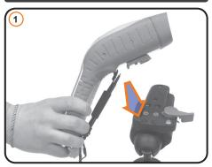
With the release lever open and pointing forwards, lower the rear of the tripod quick release plate into the tripod mounting recess.
