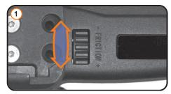
Turn the dial just enough that the IKE is fully supported (with the main lever released).
