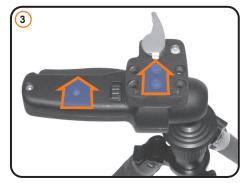
Replace the top plate so that the quick release lever faces the same direction as the main lever.
